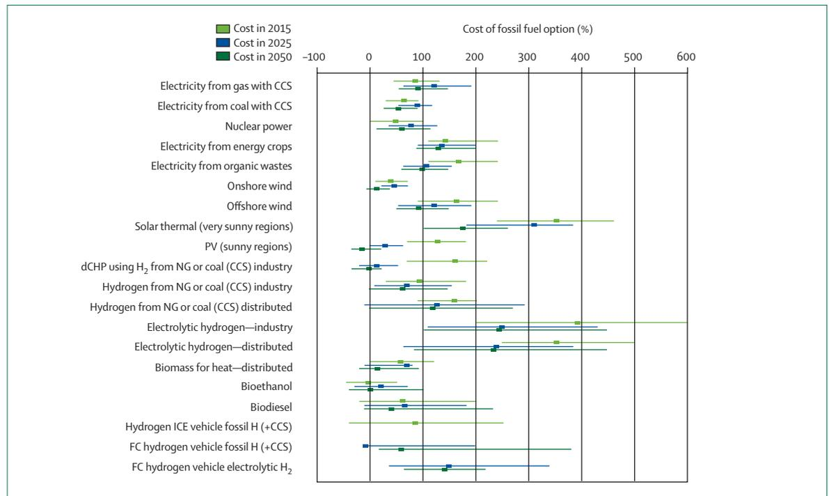
**Figure 4:** Costs of energy technologies to constrain emissions to today's levels in 2050, expressed as amount in percent by which they exceed costs of fossil-fuel alternative in 2015, 2025, and 2050<sup>9</sup>
